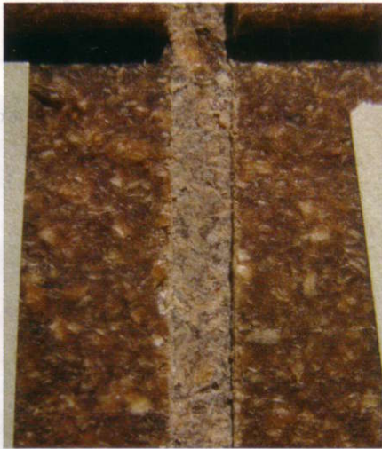
Microstructure of a typical WPC showing outer layer removed and inner material still encapsulated in plastic (x100). The microstructure of a typical WPC (x50) (Images: Tangram Technology Ltd)
