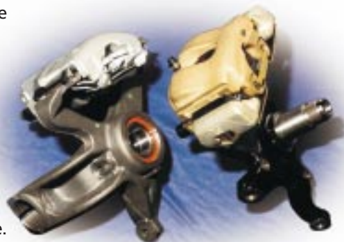
New design caliper fitted to a wheel knuckle (left) compared with an equivalent conventional two-part caliper (right)
