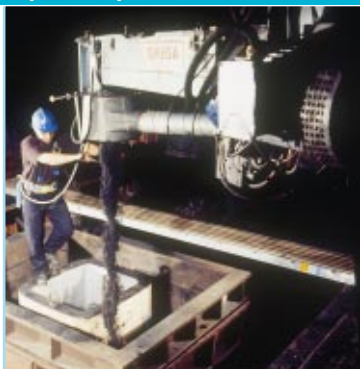
Corus Foundry's automatic mixer control system
